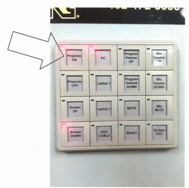
Below is the AV panel in the Gaughan Center. It is located right below the projection screen. When you arrive the Projector Off button will be red. Push the Projector on button and the projector will turn on and again please give it a few minutes to warm up and begin projecting. This is the setup in Ubuntu/Room 202 and Unity/Room 212.
